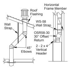
Figure 19 - 45° and 30° Offset with Wall Strap
